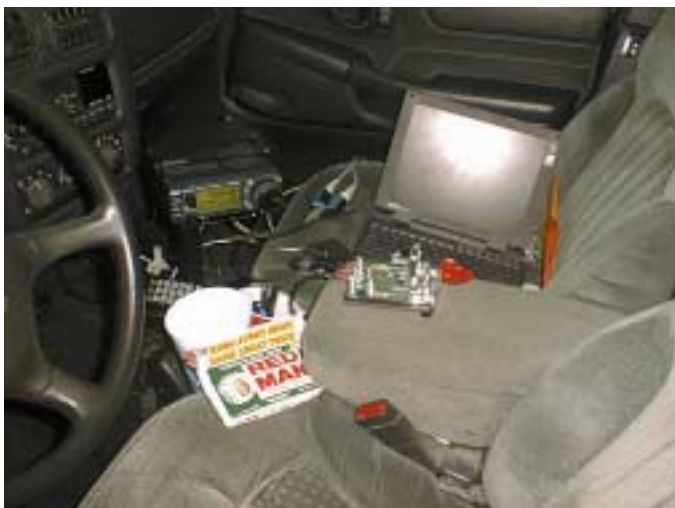
NF4A Mobile - Top Right: The 20/20 combo on the trailer hitch. Center Right: The 15 Meter Hamstick on the front bumper. Below: The operating position. The 706 was mounted on a special mount for police cars to hold their laptop...of course, there is the pack of Red Man, the official chewing tobacco of the FQP
